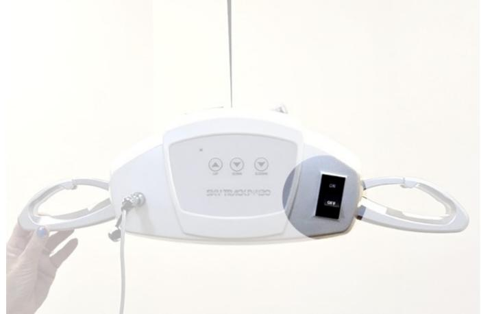
Should the emergency stop function be used in an emergency, then before the lift can be used again, it must be inspected by an authorized dealer. Once the lift has been inspected and/or repaired, then the Emergency Stop Button can be set to the "ON" position. Normal use of the lift may then proceed. Note: The lift will only charge if the Emergency stop switch is in the "ON" position. Refer to the section titled, <u>"Charging the lift"</u> for charging instructions.
