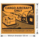
Note: All lithium ion cells and batteries shipped by themselves (UN 3480) are forbidden for transport as cargo on passenger aircraft. All packages prepared in accordance with Packing Instruction 965, Section IA, IB and II, must bear a Cargo Aircraft Only label, in addition to existing marks and/or labels.
