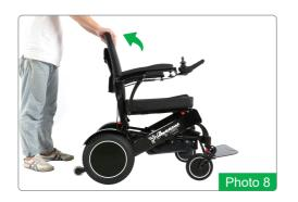
2. Continue to expand the chair into a seated position until you hear a \*CLICK\* indicating it has locked into the seated position (Refer to photo 8).
