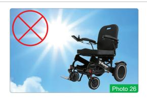
Electric walking vehicle should be placed in a place where the sun can not shine, please avoid sunlight, otherwise it is not only harmful to the battery, but also has a direct impact on the service life of plastic parts and stickers of electric walking vehicles (Refer to photo 26).
