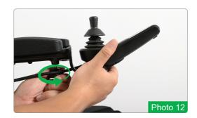
Connect the controller wire harness to the CPU wire harness. Take care the line up the pins properly as arrow tip indicate, so that they do not get bent, broken or damaged (Refer to photo 13).
