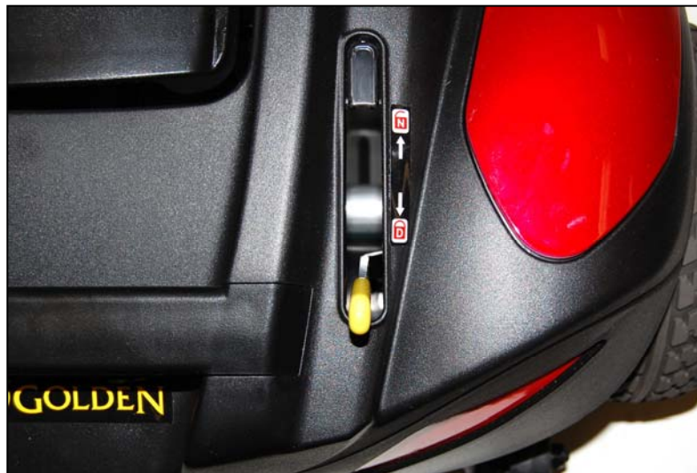
Figure 11: Freewheel Lever (Drive Position)
