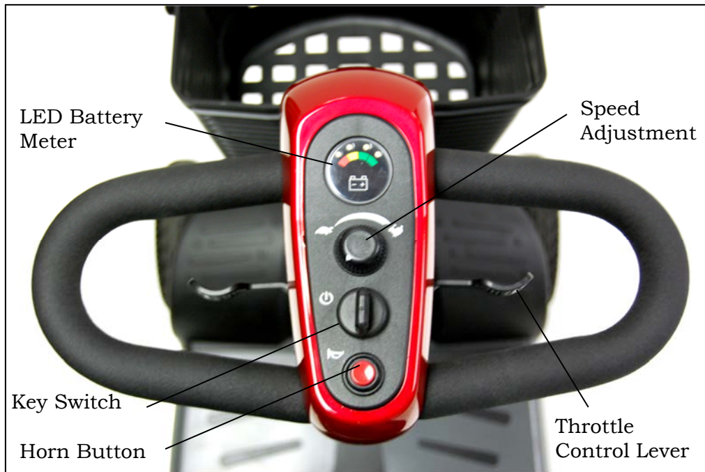
Figure 5. Buzzaround XL™ Delta Tiller Control Panel
