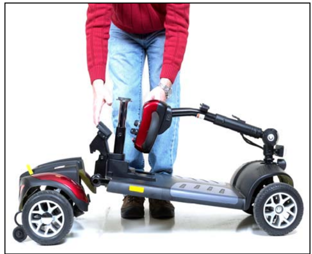
Figure 20. Connecting Frame and Drivetrain
