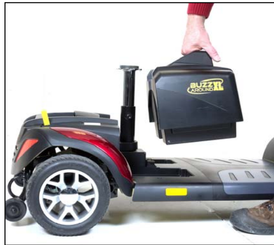
Figure 15. Removing the Battery Pack
