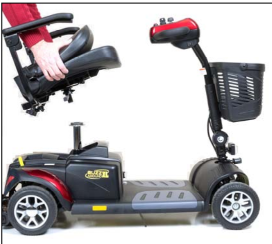
Figure 14. Removing the Seat
