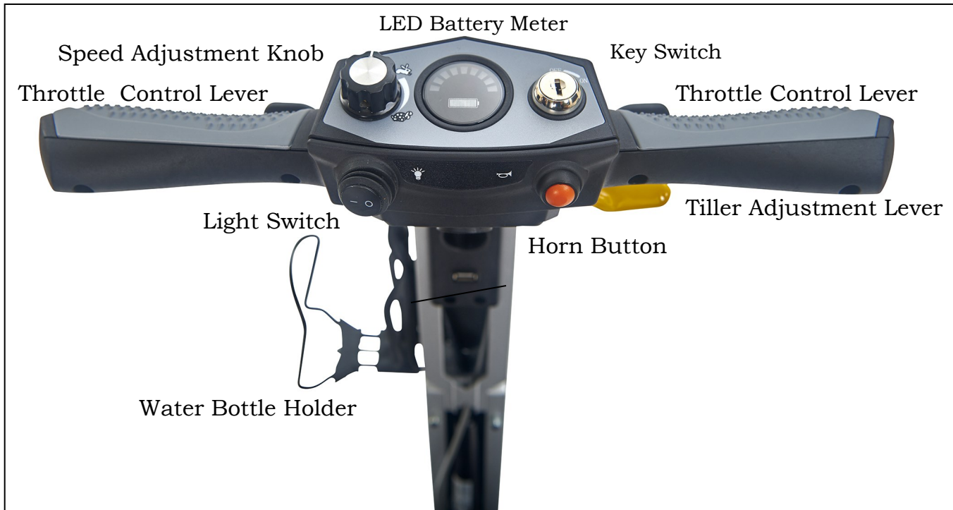
Figure 5. Carry On Tiller Control Panel
