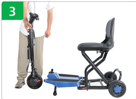
Step 3 Separate front steering post and wheel assembly from rear assembly.
