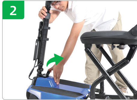
Step 2 Pull back the front end lever.
